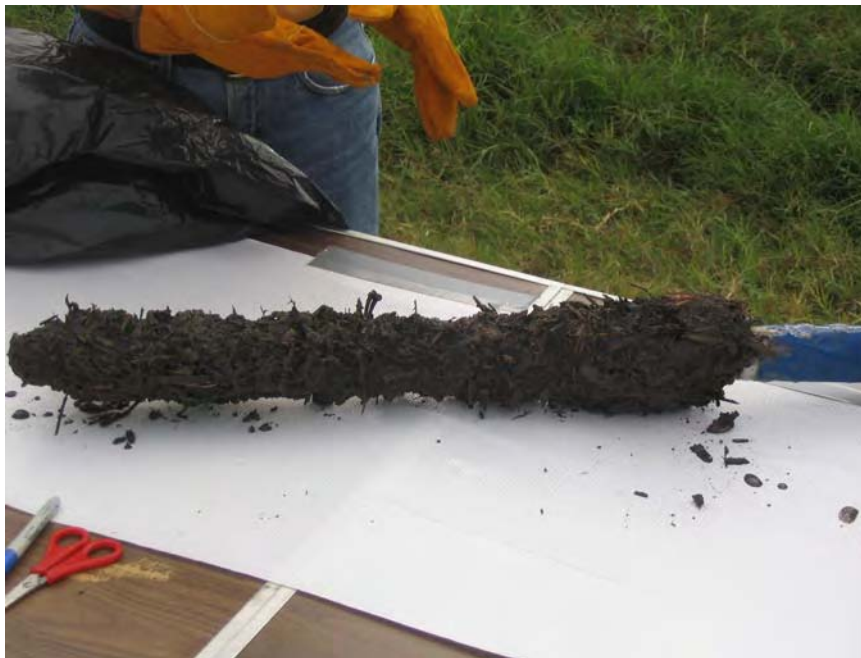
Figure 6.2 Frozen Sample of Biowall Material Collected Using Liquid Nitrogen Method at Altus AFB, Oklahoma (photo used with permission of the USEPA NRMRL/GWERD)
