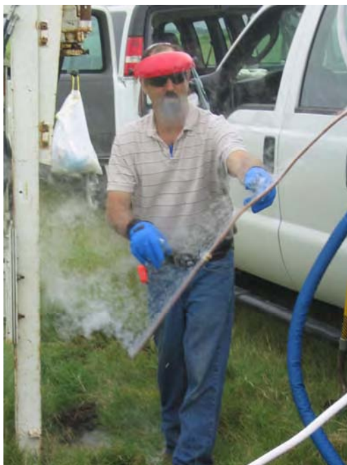
Figure 6.1 Nitrogen Sprayer from Copper Tubing to Inject Liquid Nitrogen (photos used with permission of the USEPA NRMRL/GWERD)
