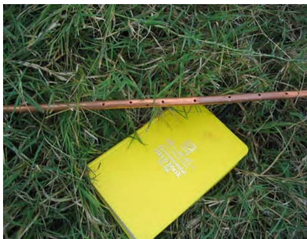
Figure 6.1 Nitrogen Sprayer from Copper Tubing to Inject Liquid Nitrogen (photos used with permission of the USEPA NRMRL/GWERD)
