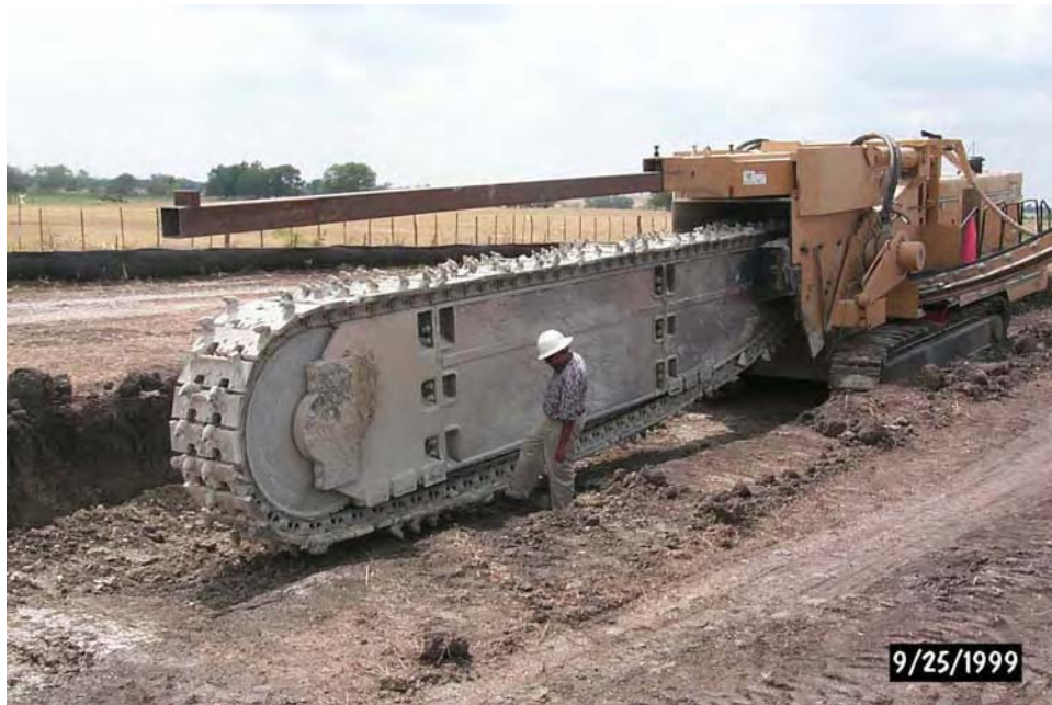
Figure 2.2 Rock Trencher Employed at NWIRP McGregor, Texas (Photo Courtesy of US Navy)
